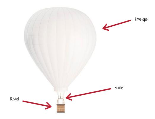
The envelope is the fabric that is attached to the basket by cables. The fabric traps hot air, which causes the balloon to rise.
