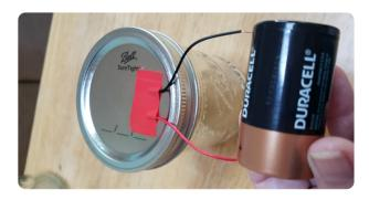
• Test the buzzer when it is sealed inside the mason jar by holding the wires to the battery and turning on the noise meter app on your smart phone.
