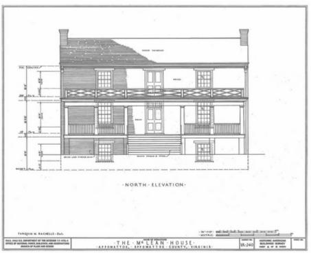
This is a photograph of the measured drawings showing the front of the McLean House. Notice how each part of the house is labeled with the materials that are to be used. For example, the roof is to be covered with wood shingles. The outside of the house is brick. It also tells the builder the type of pattern that the bricks will be laid in. Even the windows are to look a certain way. Most homes during the period of the Civil War were built of wood or brick.
