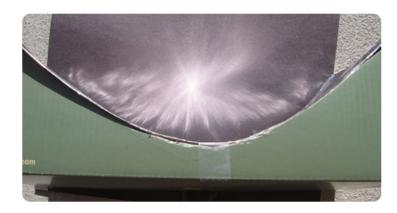
After the paper has sat in the sun for a little bit, touch the focal point carefully to make sure it is nice and hot.
