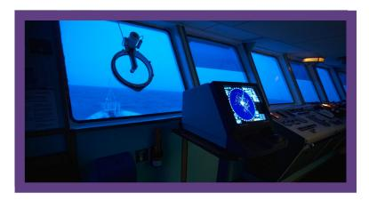
Sonar works by sending out sound waves from a submarine. It uses echoes of the sound to figure out if there are other objects around.
